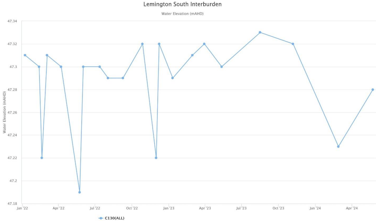
Figure 58 - Lemington South Interburden Water Elevation Trend - Q2 2024
